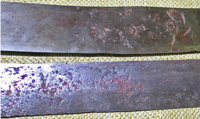
Blades from the brass- and wood-handled cutlasses above. Note the poor quality of steel available to the Confederacy.
