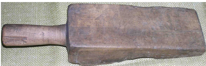
A wooden wedge with handle called a quoin was used to level the cannons when sighting.
